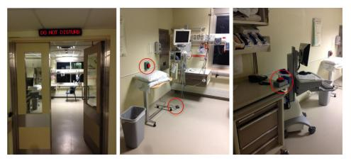
Fig. 1. The installed LED sign (left), the wall LED button and the foot pedal (center), and the desktop LED button (right).
