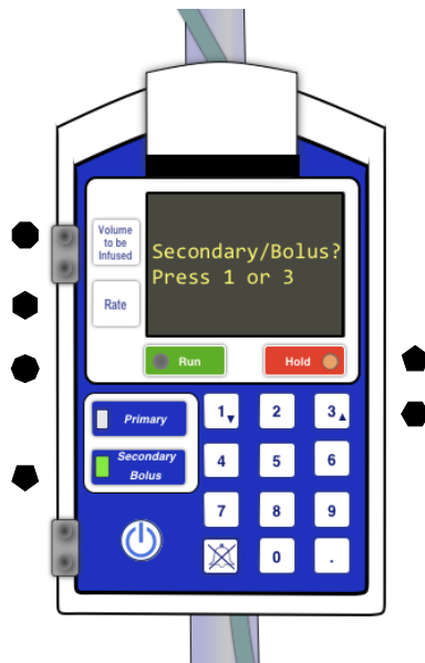
Figure 24: Administering an IV Pump Bolus: Traditional Pump Bolus Feature
